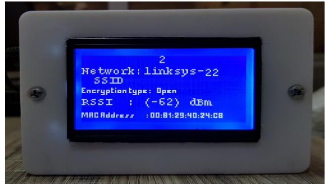
Figure 5. Displaying the Wi-Fi networks in sequence on the GLCD.
